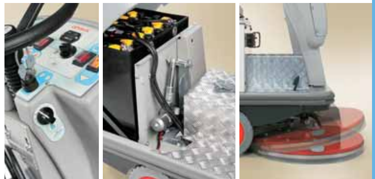
3-position knob for brush pressure adjustment, extremely effective on irregular floors. The brush head is automatically lifted and lowered by an actuator that is connected to the gear lever.
